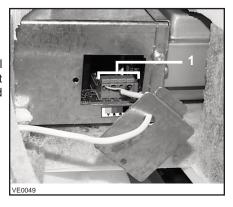
**10.** Reinstall the side door on the electrical box.
